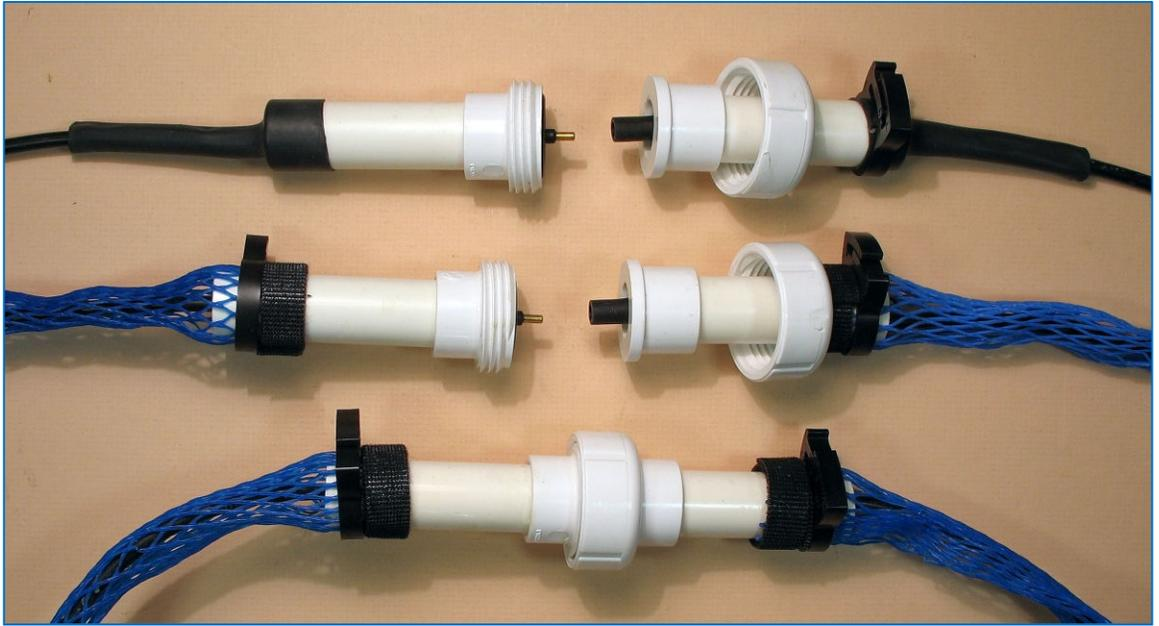
The **Model AT** is an impressed current linear anode system that permits maximum design flexibility. It consists of copper-cored titanium flat wire coated with mixed metal oxide and attached to a #14 AWG HMW/PE insulated bus wire. A flexible plastic mesh surrounds the wire pair. Individual anodes are 50 feet (15 m) long and are easily connected in the field to form a secure sealed joint. This allows the design engineer to choose a layout that is best suited for the application.
